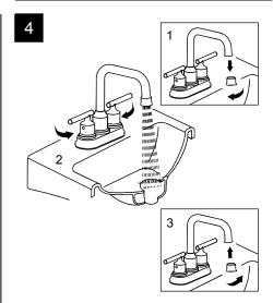
To flush debris from the plumbing system:
