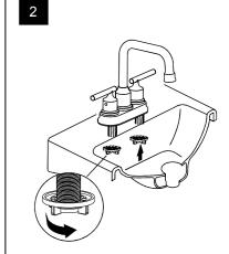
Attach the mounting nut to the hot and cold threaded mounting shanks and tighten faucet to basin.
