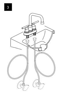
Attach supply lines (not included). Do not overtighten.
